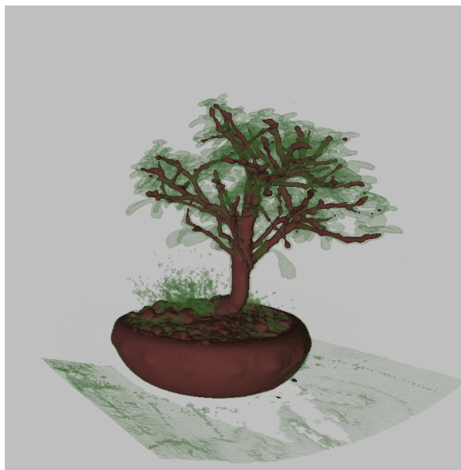
Figure 2.1: This illustration shows a CT scan of a bonsai. The leafs are visualized by direct rendering whereas the trunk and the branches are visualized using an isosurface rendering. Obviously in the direct rendering each voxel contributes to the resulting 2D image. (Source: [11])
